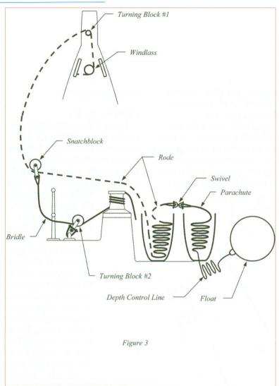
since the boat will be forereaching to leeward. Open the parachute bag and slam it, open end down, into the water; the weight of the swivel and thimble should pull the parachute out of the bag if it was properly packed. Break or cut the light threads holding the rode to the stanchion bases to allow control by the bowman. Feed the rode from its storage bag toward the bowman. Ease the bridle initially to position the snatch block halfway between midship and the bow.
