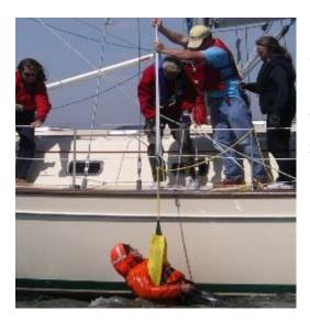
The Inflatable Lifesling is a throw bag that also works on the same principle as the standard Lifesling when inflated. After it hits the water, an automatic system inflates it to make a combination life ring/hoisting device.
